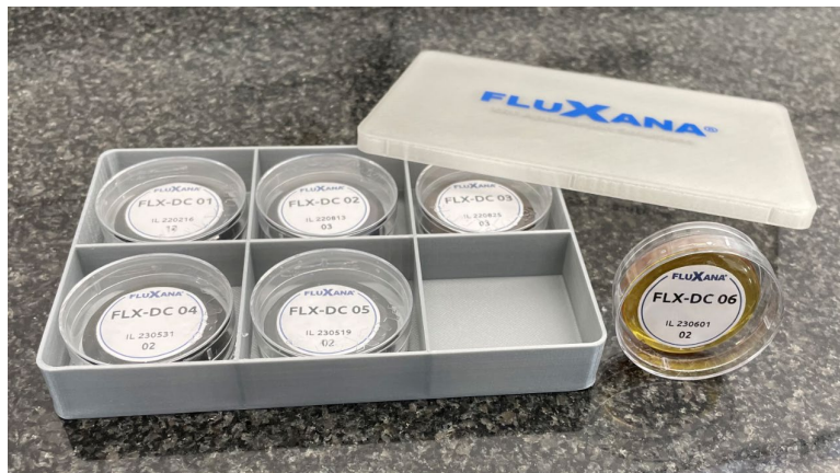
Fig. 3 Universal drift monitor set FLX-DC consisting of 6 samples FLX-DC 01 to FLX-DC 06.
