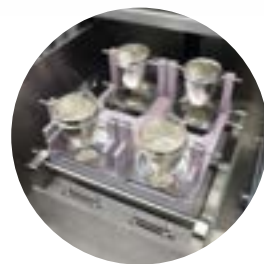
Equal temperature distribution on all 4 samples
