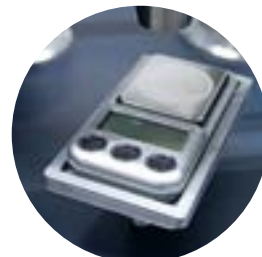
Additional scale for sample weighing
